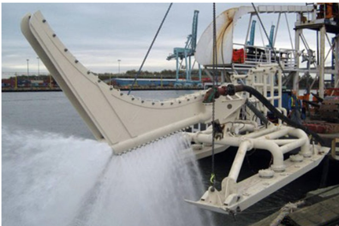
Figur 3.12 Mod-Jet/Sea Venture strømkabelslæde (kilde: https://eta-ltd.com/jetting-sleds-for-subsea-power-cable-laying/ )
