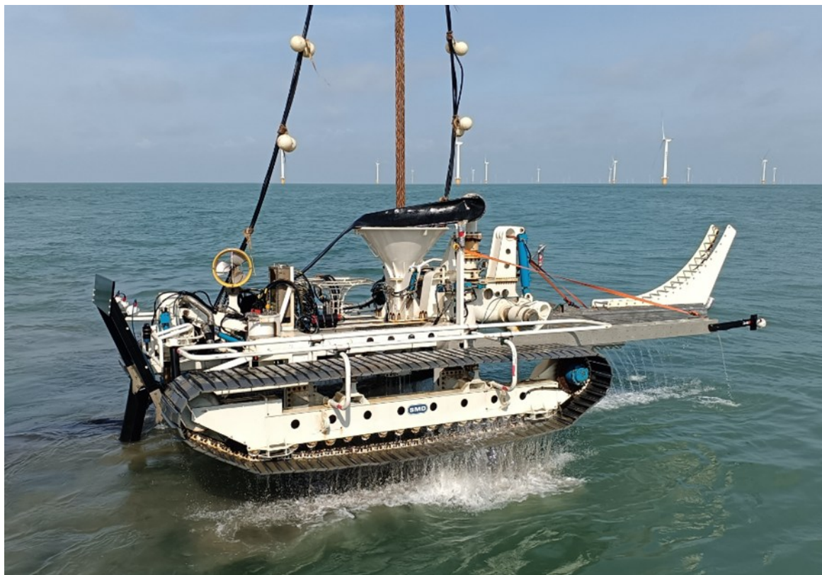
Figur 3.13 Lavvandsgravemaskine (Shallow Water Trencher) (kilde: https://www.smd.co.uk/blog/may-2023-smds-shallow-water-trencher-the-story-so-far/ )
